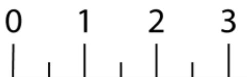
Many thermometers have numbered marks every ten degrees with unnumbered marks for the degrees in between. That type of thermometer would not be appropriate for your candidates to measure the temperature of a workplace. An appropriate thermometer would have each degree marked and numbered.
